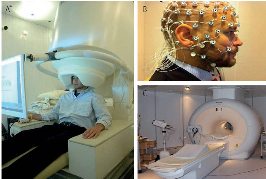
A – Magnetoencephalography (MEG), B – Electroencephalography (EEG), C – Functional magnetic resonance imaging (fMRI) (Wikipedia.org).
